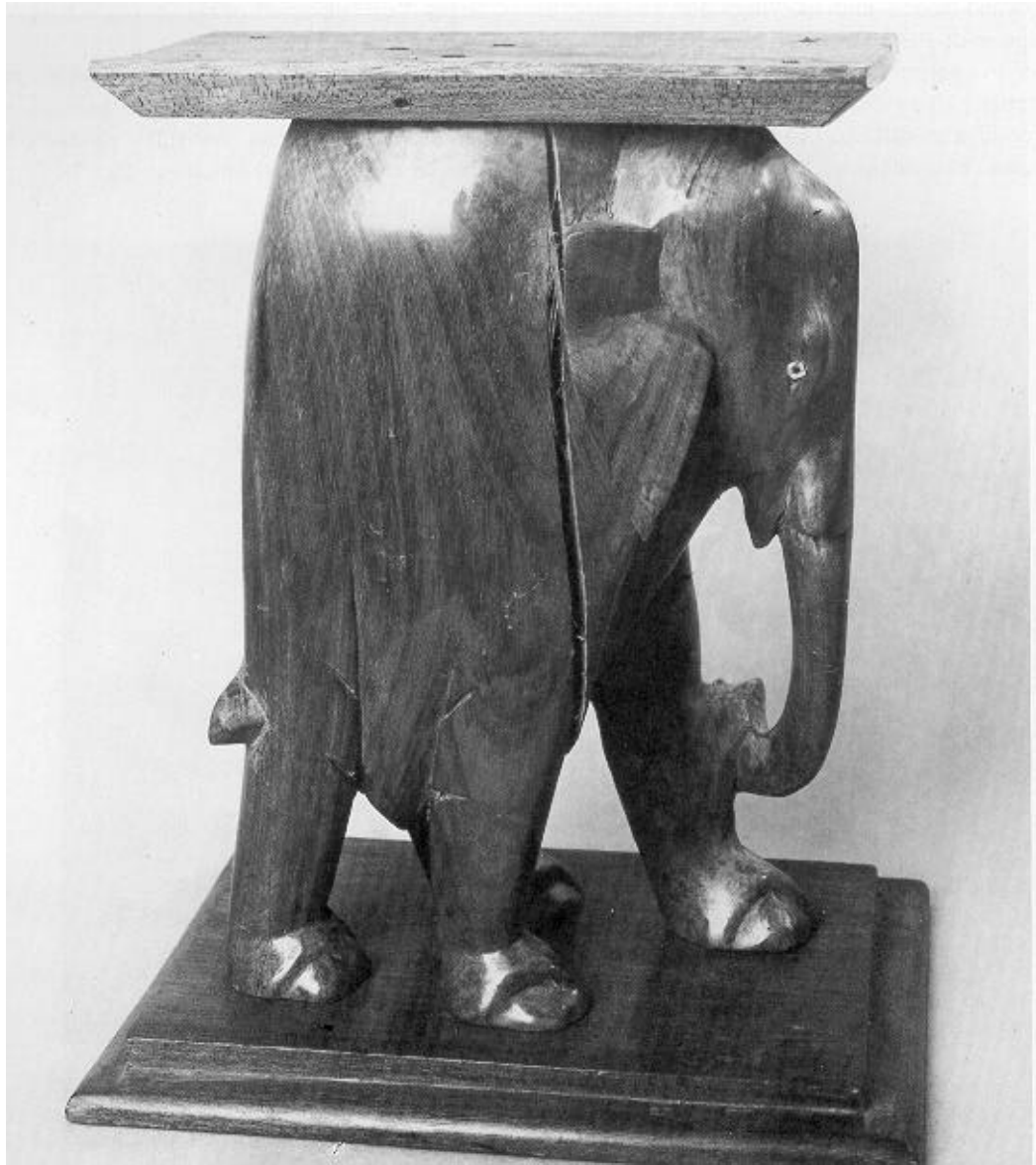
Figure 6.--Many of the carvings imported from tropical countries develop the serious checks and splits shown above while they dry out in the arid environment of our heated and air-conditioned stores, offices, and homes.
