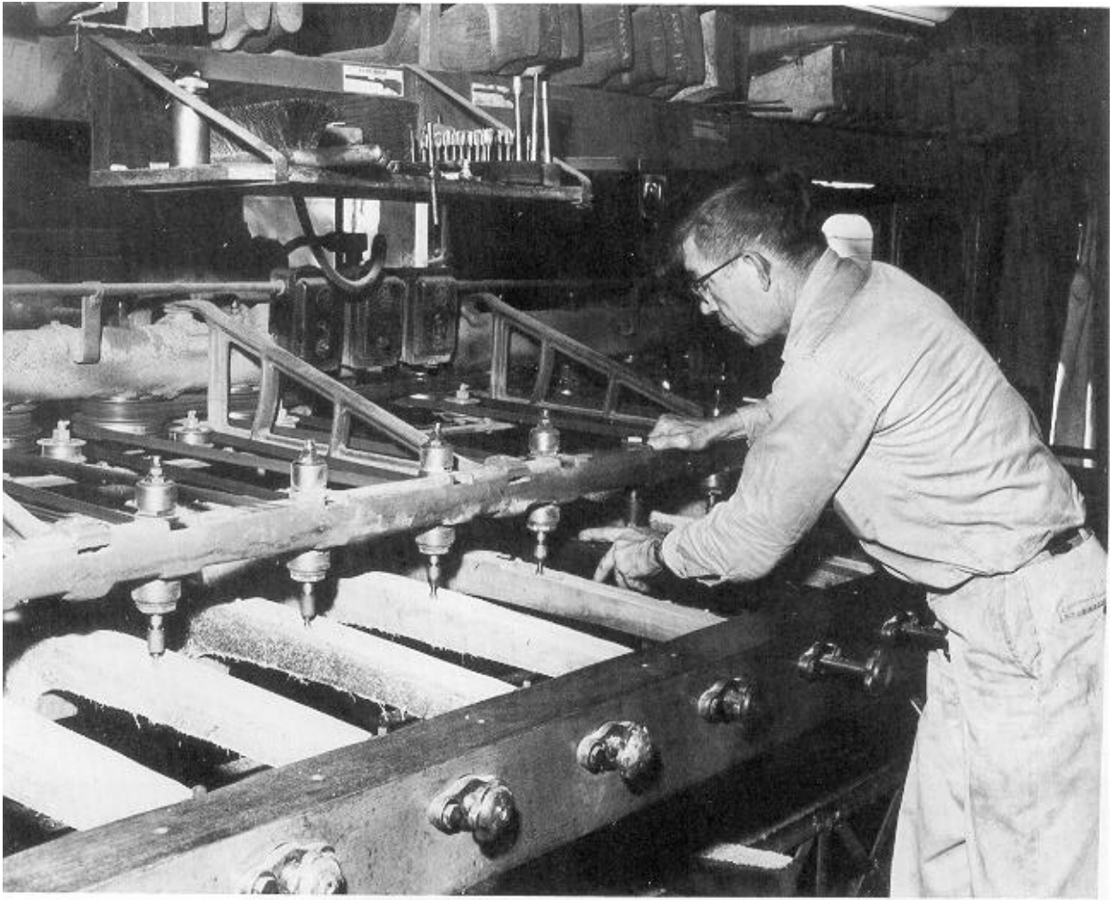
Figure 5.--A master stockmaker shapes and inlets sporter rifle stocks from green, fresh-cut walnut blanks. The stocks will be PEG-treated and kiln-dried to 6 percent moisture content.
