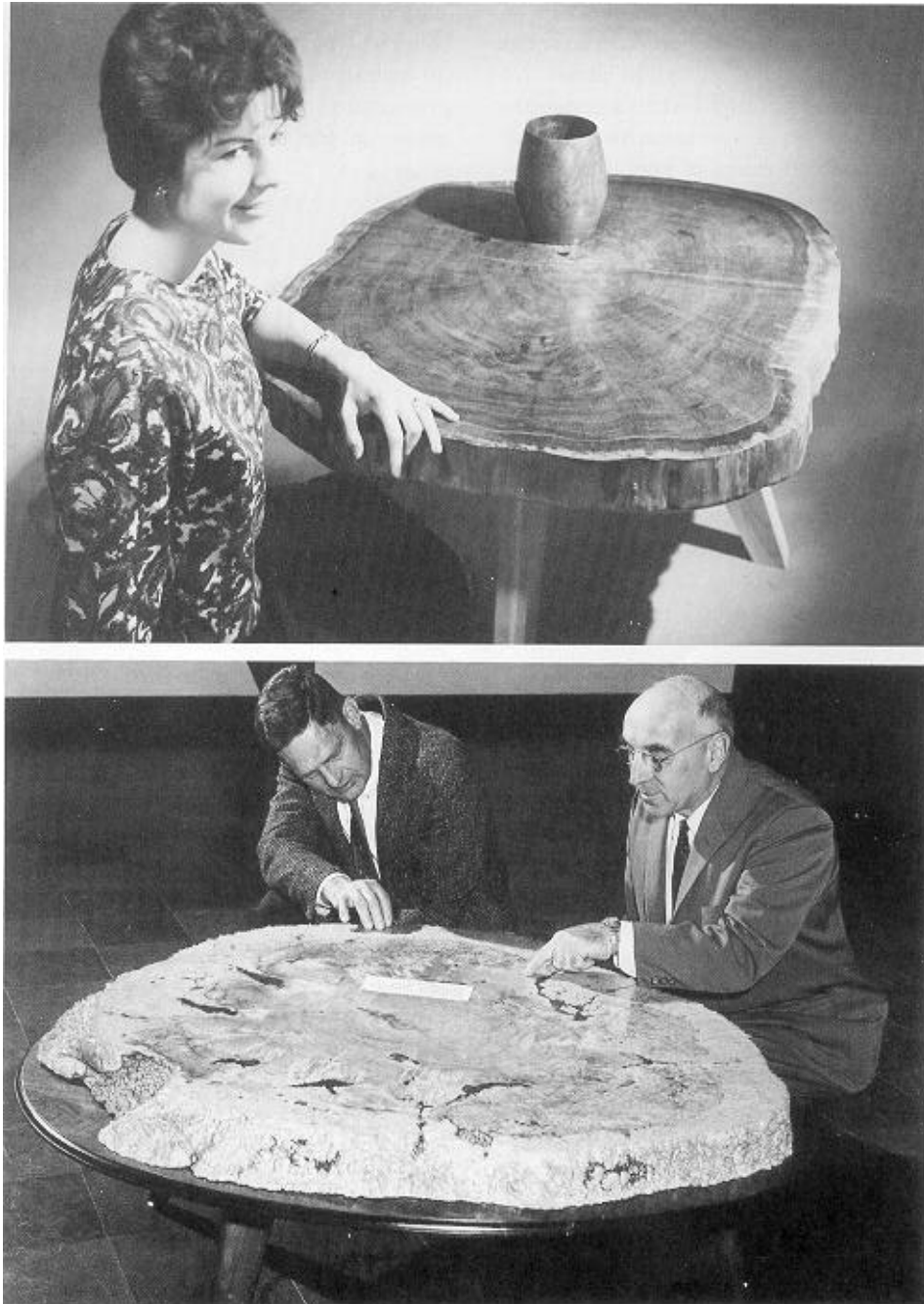
Figure 1.--Stabilized disks. Top, PEG-stabilized tabletop, 38-inch diameter, cut from butt of 784-year-old redwood; bottom, king-size PEG-stabilized cross section through large boxelder burl.
